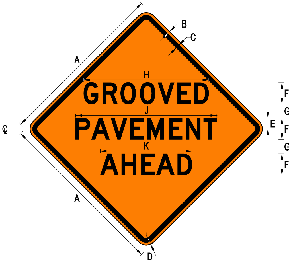
W20-V14 GROOVED PAVEMENT AHEAD
