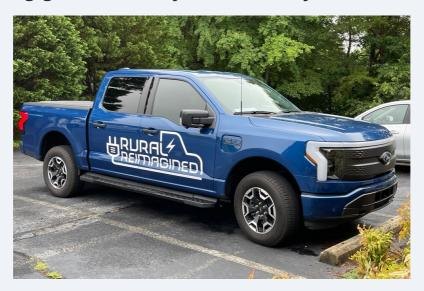
Pittsylvania County Public Works has an all-electric F150 Lightning on loan through a program with Virginia Clean Cities and Rural Reimagined. It has a charger that can be plugged into a standard 120V plug and a range of about 230 miles on a full charge.
